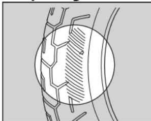
Inspect the tyres for signs of abnormal wear on the contact surface.
