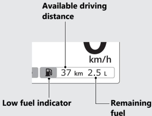
After refuelling more than the reserve amount, the display returns to normal when the electrical system has been on for about a minute.
