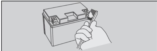
4. After cleaning, reinstall the battery. The battery has a limited life span. Consult your dealer about when you should replace the battery. Always replace the battery with another lithium-ion (li-ion) battery of the same type.
