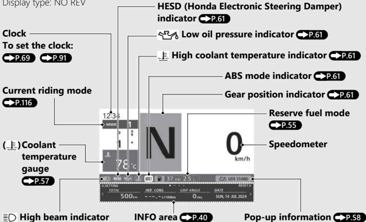
The tachometer is not displayed when NO REV is selected.
