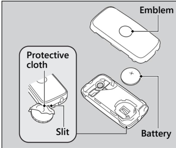
2. Replace the old battery with a new one with the positive ⊕ side facing up.
