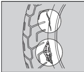
Inspect the tyres for cuts, slits, or cracks that expose fabric or cords, or nails or other foreign objects embedded in the side of the tyre or the tread.
