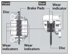
Brakes Inspecting the Brake Pads
