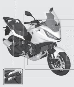
Fuse puller, Hex wrench, Standard/Phillips screwdriver, Screwdriver handle P.224 Rear brake fluid reservoir P.250 Front brake fluid reservoir P.250 Front brake lever P.260 Main fuse & ABS main fuse P.292 NT1100A FI fuse & Main 2 fuse ►P.293 NT1100D FI fuse & Main 2 & DCT main fuse P.294 Fuse box & ABS FSR fuse P.291 Battery P.243 Coolant reserve tank Rear brake pedal
