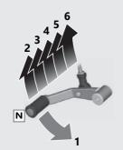
If you put the vehicle in gear with the side stand down, the engine will shut off.
