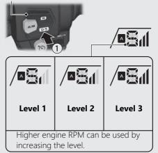
The selected level is maintained even when the ignition switch is turned to the  $\bigcirc$  (Off) position, or transmission is switched to out of S mode.
