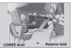
If the coolant level is dropping noticeably or the reserve tank is empty, you likely have a serious leak. Have your vehicle inspected by your dealer.
