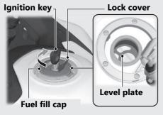
Do not fill with fuel above the level plate. **Fuel type:** Unleaded petrol only **Fuel octane number:** Your vehicle is designed to use Research Octane Number (RON) 91 or higher.
