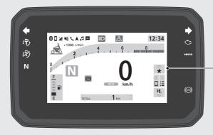
Do not operate the display functions for a long time with the engine stopped. It may result in a low (or dead) battery.
