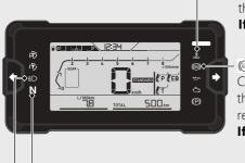
**■E**High coolant temperature indicator Comes on when the ignition switch is turned to the (On) position.
