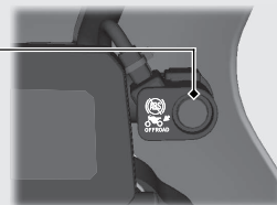
ABS function on both wheels is on.
