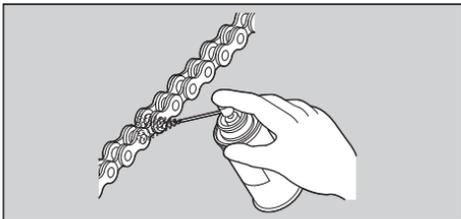
Never use petrol or low flash point solvents for cleaning the drive chain.
