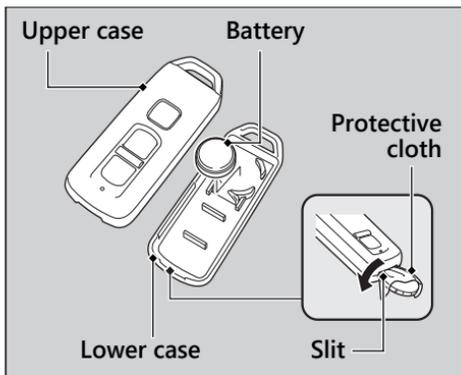
2. Replace the old battery with a new battery with the negative  $\ominus$  side facing up.
