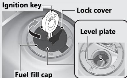
Do not fill with fuel above the level plate.
