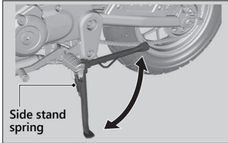
1. Check that the side stand operates smoothly. If the side stand is stiff or squeaky, clean the pivot area and lubricate the pivot bolt with clean grease.
