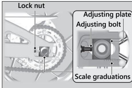
**Drive Chain ► Adjusting the Drive Chain Slack**
