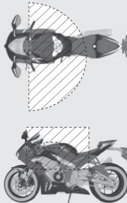
Anyone can operate the ignition switch and start the engine if your Honda SMART Key is within operating range of your vehicle, even if you are on the other side of a wall or window. If you are away from your vehicle but your Honda SMART Key will still be within the system's operating range, deactivate the Honda SMART Key system.
