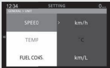
If you want to select "L/100km" or "km/L" for fuel consumption, "km/h" must be selected in the "SPEED" menu in advance. When "mph" for speed is selected, "mile/gal" or "mile/L" can be selected.
