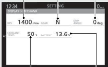
**Coolant temperature**    **Battery voltage**
