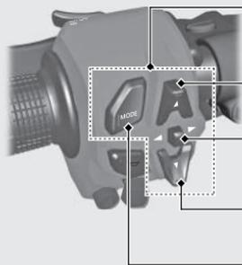
These switches are used for operating and setting the display. ➔ P.33
