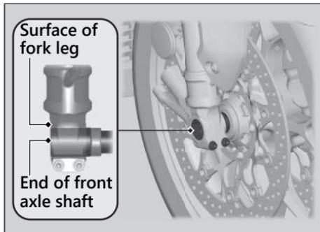
4. Tighten the right axle pinch bolts to hold the axle.
