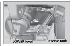
If the coolant level is dropping noticeably or the reserve tank is empty, you likely have a serious leak. Have your vehicle inspected by your dealer.
