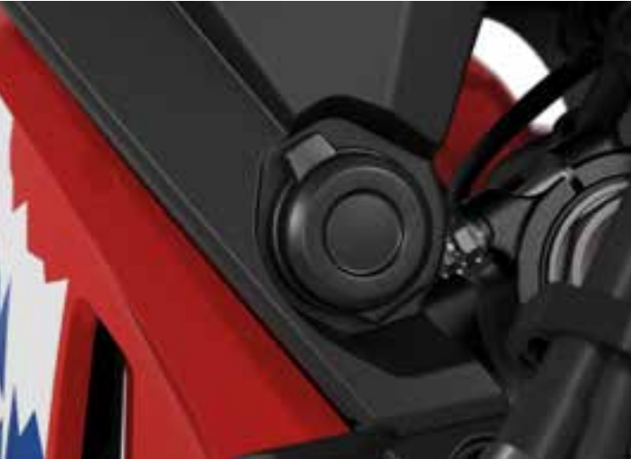
12V SOCKET 08U70-MKS-E00 Installed on the control panel, this 12V Socket is ideal to power or charge electrical equipment.
