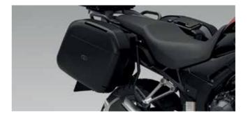
PLASTIC PANNIERS SET 08L70-MGZ-080 Set of two aerodynamically shaped panniers fully integrated with the design of the CB500X. Stay and key system sold separately.
