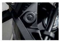
12V SOCKET 08070-MKP-D80 12V Power Socket allows you to power or charge electrical equipment directly from the bike.
