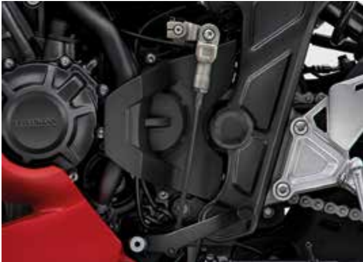
QUICK SHIFTER 08U72-MKN-D50 By measuring the intensity of the shifting input, the quick shifter enables the rider to change gear without the need to operate the clutch lever or shut the throttle. The system aids upshifting, maximizing the riding experience. Not compatible with E-Clutch versions.
