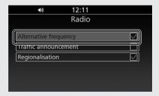
3 Select [Alternative Frequency], and then press or **ENT** switch to select (enable) or deselect (disable) the function
