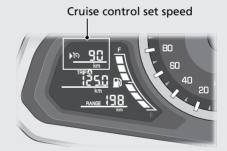
Each quick tap (brief push and release) on either side will change your speed by 1 km/h or 1 mph (depending on mileage meter set unit).
