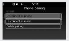
[Rider HS pairing] / [Passenger HS pairing] Select [Disconnect], and then press or ENT] switch.
