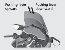
Turning the ignition switch to **O** (Off) will automatically lower the windscreen to its original position.
