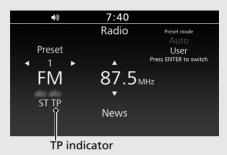
When a radio station capable of providing traffic information is selected, the "TP" indicator will appear on the screen that traffic reports can be received from this station. The system will automatically switch to a traffic announcement if a traffic information is received.
